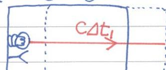
$$l + v\Delta t_1 = c\Delta t_1$$
