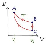
cycle as shown in the figure. The heat engine starts from state A, to state B and state C, then returns to the original state A. The first process  $A \to B$  is isothermal at temperature T from a smaller volume  $V_1 = v$  to the larger  $V_2 = 8v$ ; the second process  $B \to C$  occurs at constant volume and the third process  $C \to A$  is adiabatic. Find the efficiency  $\epsilon$  of the heat engine in terms of T, v and the ideal-gas constant R.
