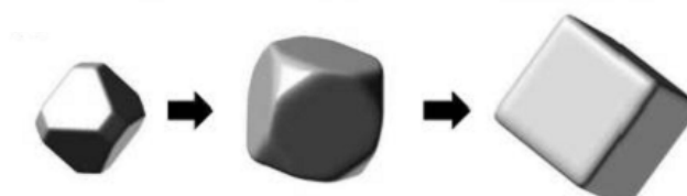
Figure 2.29 The overall shape evolution of the \text{Fe}_3\text{O}_4 nanoparticles[52]
