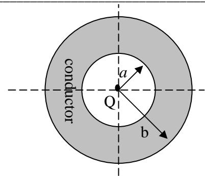
Ans: The surface normal at  $R = a$  is  $-\hat{a}_R$  and that at  $R = b$  is  $-\hat{a}_R$ . The electric flux density at  $R = a$  is  $\vec{D} = \frac{Q}{4\pi a^2} \hat{a}_R$  and that at  $R = b$  is  $\vec{D} = \frac{Q}{4\pi b^2} \hat{a}_R$ . According to  $\rho_s = \hat{a}_n \cdot \vec{D}$ , the surface charge density at  $R = a$  is  $-\frac{Q}{4\pi a^2}$  and that at  $R = b$  is  $\frac{Q}{4\pi b^2}$ .
