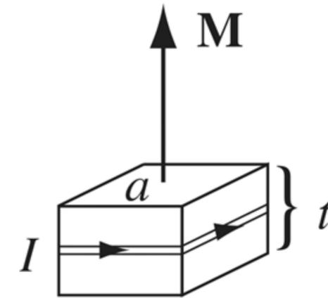
Consider a thin slab of *uniformly* magnetized material, with the dipoles represented by tiny current loops.
