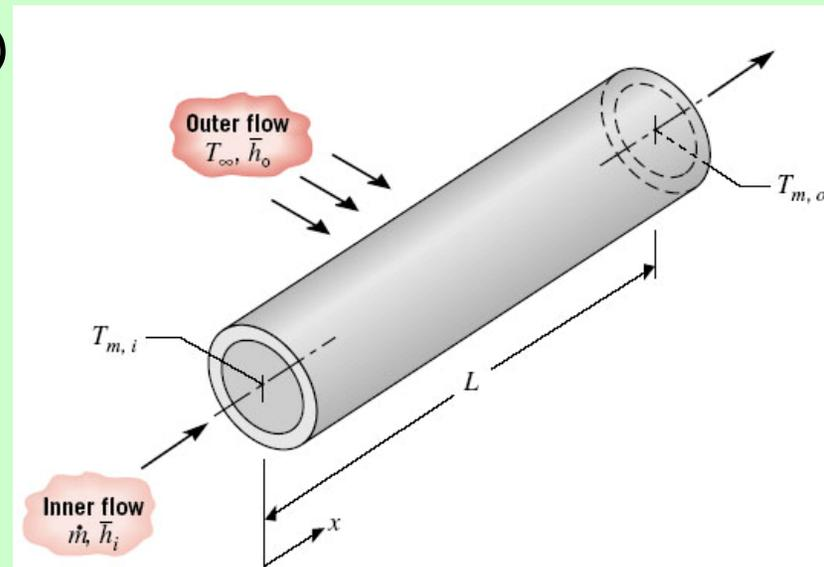
**FIGURE 8.8** Heat transfer between fluid flowing over a tube and fluid passing through the tube.
