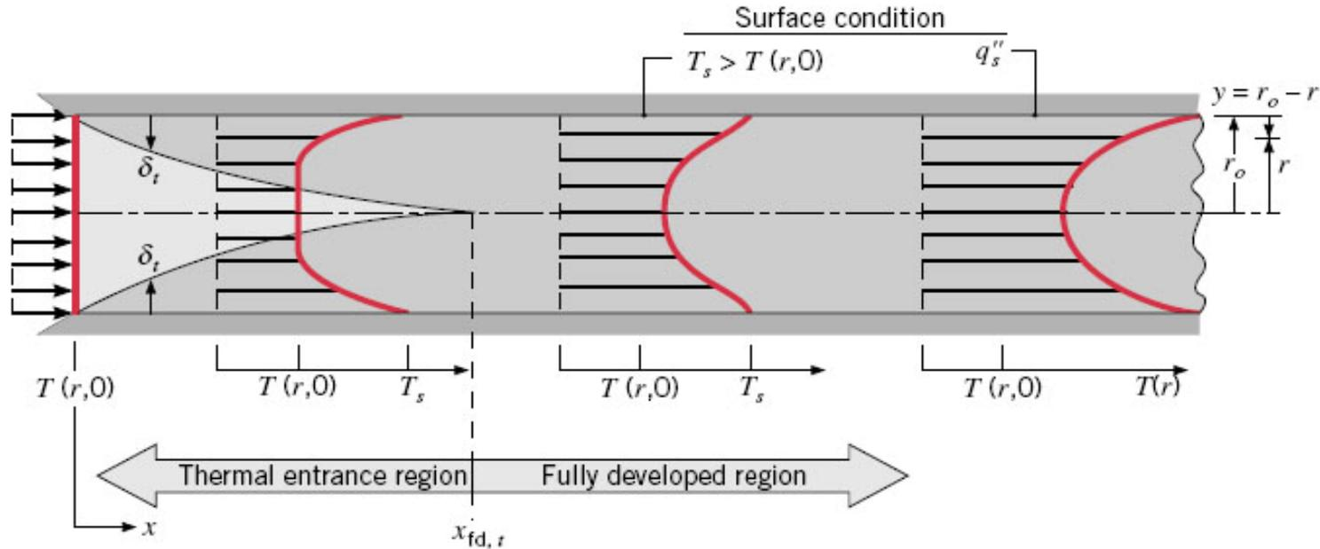
**FIGURE 8.4** Thermal boundary layer development in a heated circular tube.
