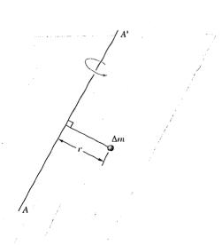
consider now a mass m, the sum of  $r_1^2 \triangle m_1$ +  $r_1^2 \triangle m_1$  +  $\cdots$  is the moment of inertia of the mass with respect to AA'
