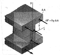
where k is a constant, y is the distance from  $\triangle A$  to an axis passing through the centroid of the section, this axis is known as neutral axis of the section [will be shown in mechanics of materials]
