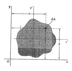
note that the first integrals with respect to centroidal axes are zero
