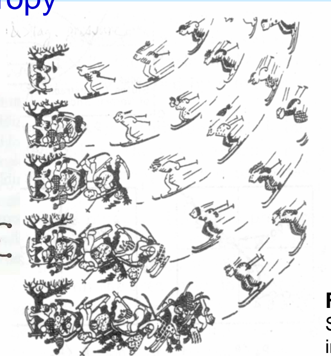
FIG. 5.20. Metaphorical shock propagating into a flowing medium which has been suddenly brought to rest. (Reprinted courtesy R. Courant and K. O. Friedrichs, Supersonic Flow and Shock Waves , Interscience Publishers, New York, copyright 1948.)
