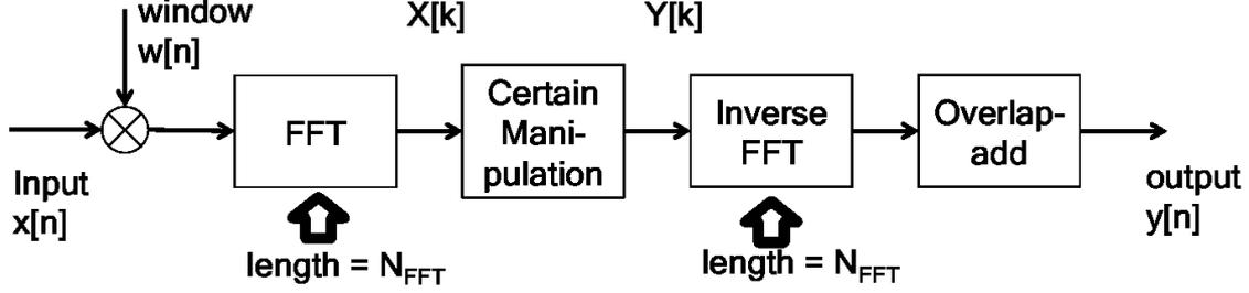
Figure 1: A general block diagram of OLA analysis and synthesis system
