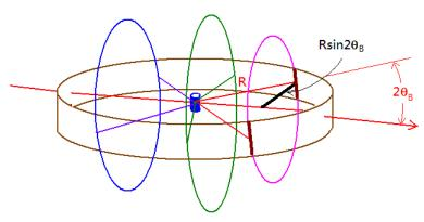
The film receives a greater proportion of a diffraction cone when the reflection is in the forward or backward direction than it does near  $2\theta = \frac{\pi}{2}$
