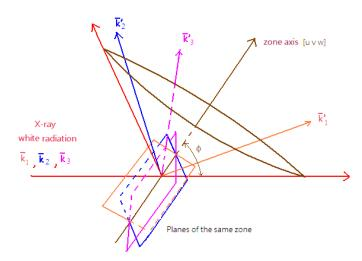
All the diffracted beam directions  $\hat{S}_1', \hat{S}_2', \hat{S}_3' \cdots \hat{S}_i'$  are on the same cone surface.
