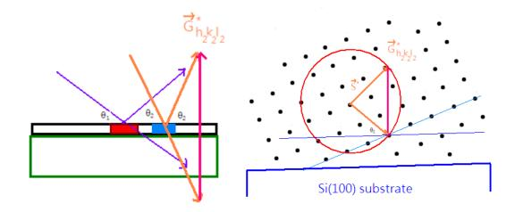
This is equivalent to at least one crystal with  $(h_2k_2l_2)$  plane normal also in parallel with the Si(100) surface normal.
