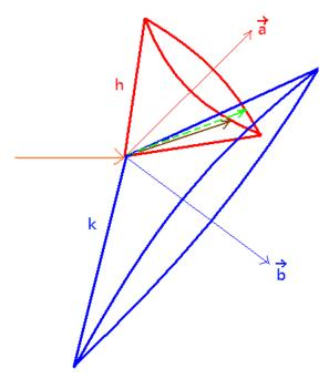
The 1st and 2nd conditions are simultaneously satisfied only along lines of intersection of cones.
