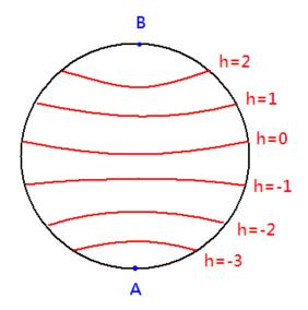
The projection of diffracted beams for h = 0 is a great circle if the incident beam direction is perpendicular, i.e.  $\vec{S} \perp \vec{a}$ .
