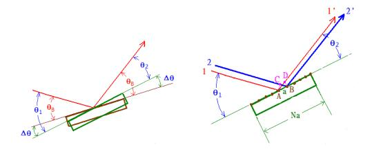
When the reflecting planes make an angle  $\,\theta_B$  with the incident beam, the Bragg law is satisfied and the intensity diffracted in the direction  $\,2\theta_B$  is maximum.
