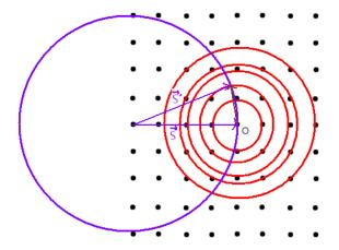
$\vec{S}'$  forms a cone resulting from the intersection between Ewald sphere and the spherical reciprocal lattice.
