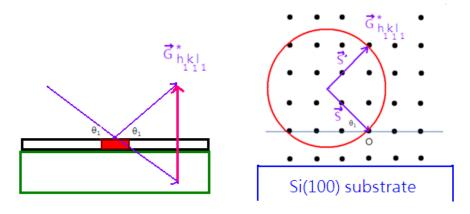
Rotate the incident beam at until  $\vec{G}_{h_1k_1l_1}^*$  meets the diffraction condition at  $2\theta=2\theta_1$
