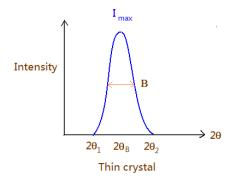
integrated intensity =  $I_{\text{max}} \cdot B$ , where B is the width at  $\frac{I_{\text{max}}}{2}$
