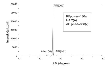
A large number of grains with AlN(002) surface normal in parallel to Si(100) surface normal, but small amount of grains of
