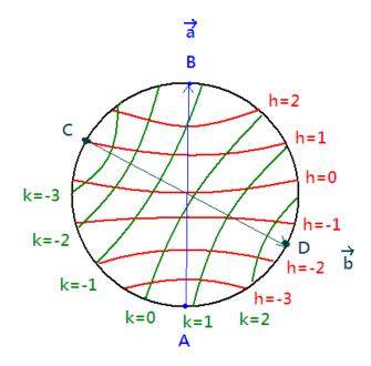
The lines of intersection of cones are labeled as (h, k)
