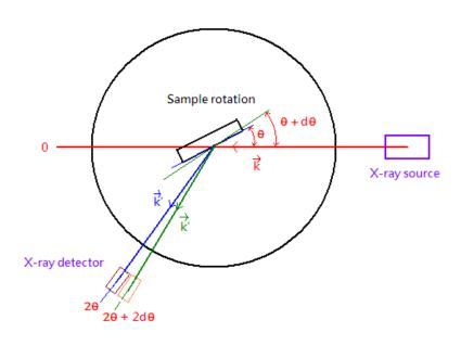
If a new material is deposited on Si(100) and put on the substrate holder in the diffractometer set-up,  $\vec{k}' - \vec{k}$  is always parallel to the Si(100) surface normal.
